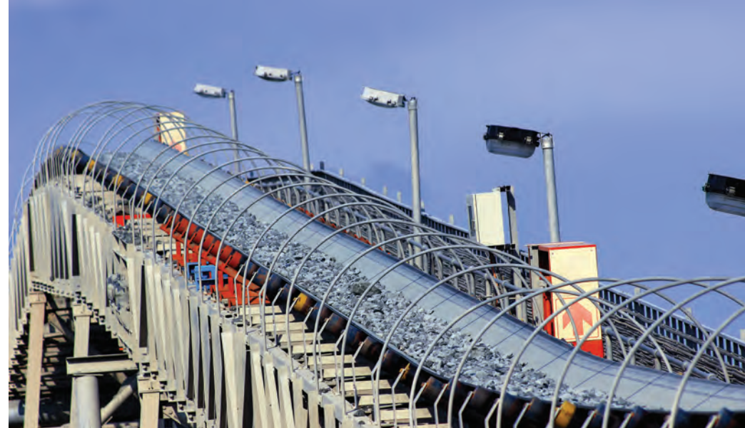
Conveying coarse kimberlite for additional size reduction
